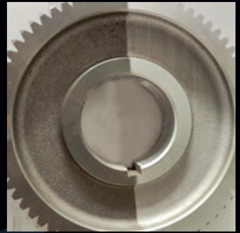
oxidation layer removal
